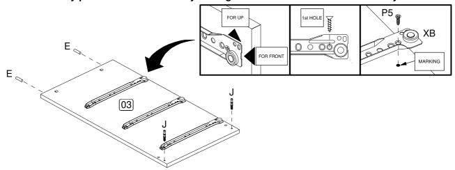
**Step 2:** Attach the metallic slide (XA) to the left panel (2) using hadware part P5. Insert hardware part E using a small mallet (not provided) and the part J using screwdriver (not provided).
