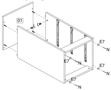
**Step 6:** Secure the back panel (10) using hardware part N and a small mallet (not provided). **DO NOT use any power tools as this may damage the frame and will invalidate any claim.**
