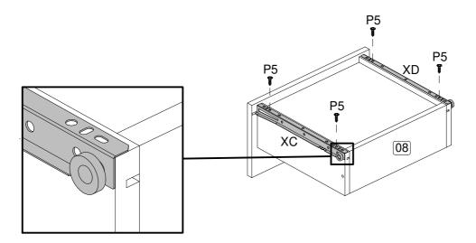
**Step 11:** Insert the drawers on the metallic slide as shown bellow.
