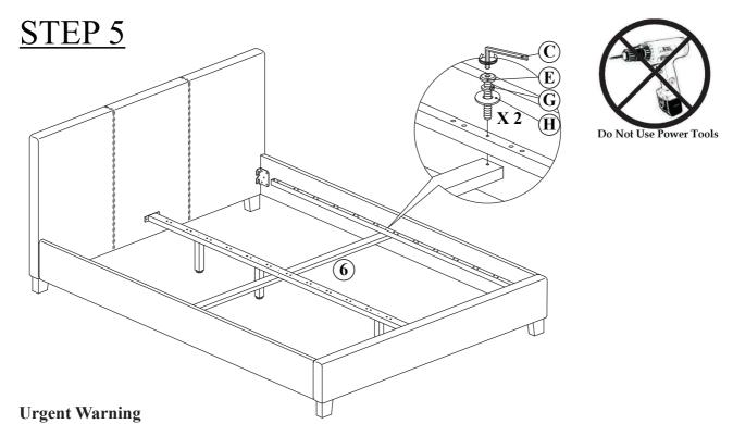
When correctly adjusted the centre support legs on this product should be raised by 5mm from the floor with the added weight of the mattress and bedding. This bed may fail if it is used on a wooden floor **WITHOUT** the use of non slip pads on all support legs and bed posts If the bed is to be moved, carefully lift the product rather than dragging to ensure that the centre legs do not become twisted and buckle.
