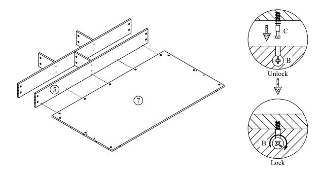
Attach the Headboard Left Panel (2) and Headboard Right Panel (3) to Headboard Center Panel (4) and Headboard Bottom Panel (5) and Headboard Front Panel (7) by screwdriver (not provided). **DO NOT** use any power tools as this may damage the frame and will invalidate any claim.
