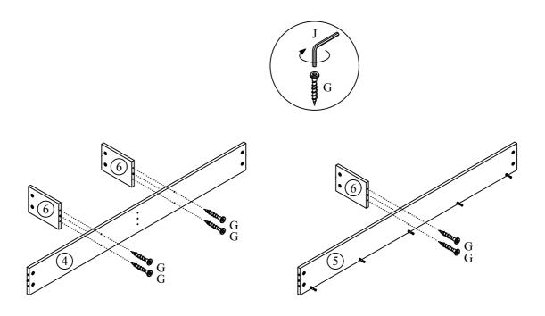
Attach the Headboard Divider Panel (6) to Headboard Center Panel (4) by screwdriver (not provided). **DO NOT** use any power tools as this may damage the frame and will invalidate any claim.
