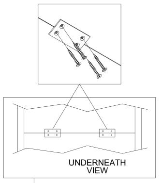
Affix metal plates to the underside of the mattress bases with fixings and screwdriver provided.
