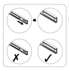
Pull slide to the front of the drawer runner track when fitting drawers. Lift or depress plastic locator if removing drawer.
