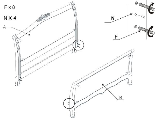
Step 2 - Locate the side rails onto the threads protruding from the headboard. Locate the washer & Nut (G) onto the threads and secure by hand at first. Tighten evenly using the open ended spanner (Provided).
