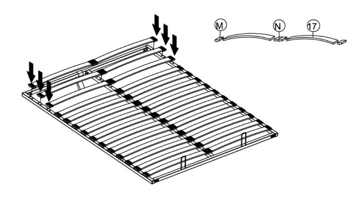
Step 7: Assemble the bed base on the right & left hydraulic frame starting from'1'to'3'as shown with HardwareH,X,R&W,and fix the support leg (16) to the bed base by Hardware G,X&R as shown .
