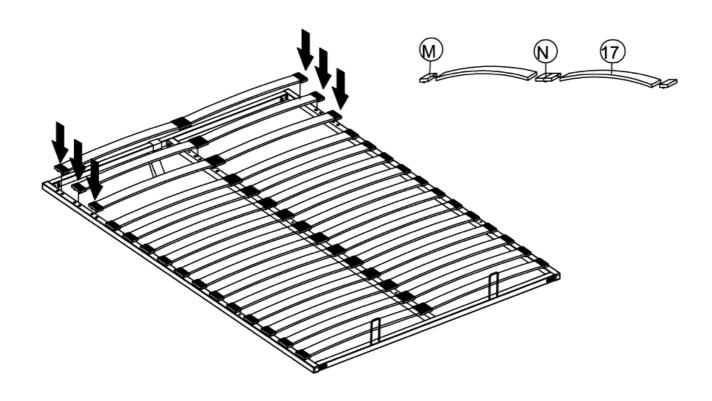
Step 7: Assemble the bed base on the right & left hydraulic frame starting from'1'to'3'as shown with HardwareH,X,R&W,and fix the support leg (16) to the bed base by Hardware G,X&R as shown .
