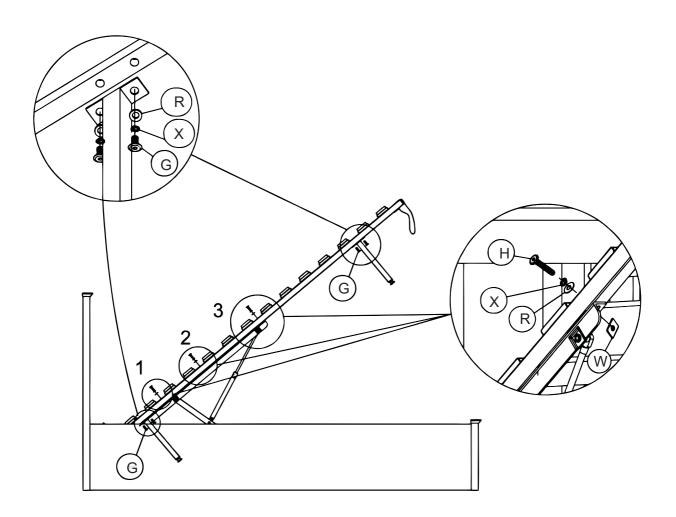
Step 8: Adjust the bed base making sure that the distance to the footboard is approximately 15mm to above . Tighten all bolts and screws now.
