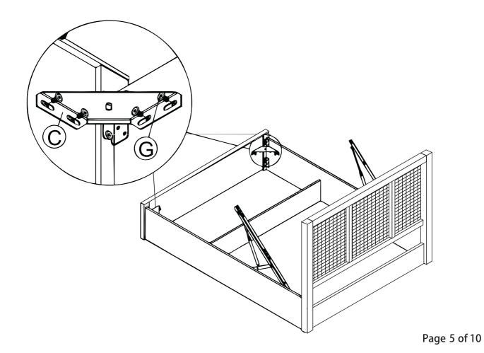
Step 5: Join together all the bed base parts (11),(12),(13) and (14) using hardware parts S,X & R and also slide part P onto Part 14 before bolting together. Attach the centre rail(15) with Metal Frame by
