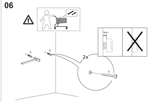
As wall materials vary, screws for fixing to wall are not included. Please contact your DIY or hardware store for advice on the correct type of screws/wall plugs for your type of wall.
