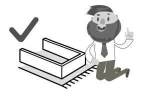
Never drag or push the pieces across a hard or stone floor as this will cause damage to the joints. Use a carpet or a rug for extra care.
