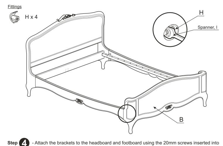
4 - Attach the brackets to the headboard and footboard using the 20mm screws inserted into the pre-drilled pilot holes. Tighten using a crosshead screwdriver.
