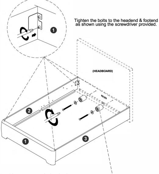
Fix the rubber stoppers to the headend as shown using the screwdriver provided.
