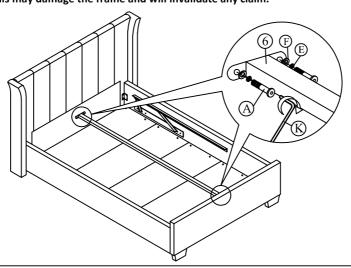
Step 8 : Unscrew the Pre-attached hex-nut of gas spring (11) and attach it back again as shown. Please fully tighten the nut.
