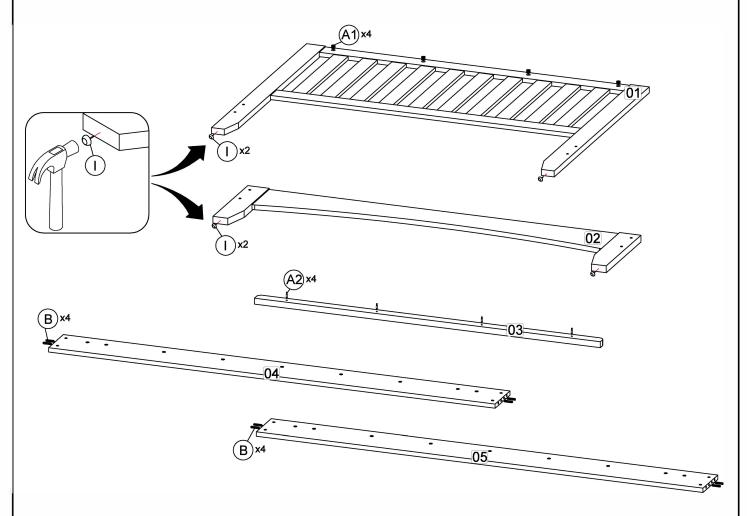
Step 2: Attach headboard top tray panel (3) to headboard panel (1) by using hardware A1 and A2 with a screwdriver (not provided).DO NOT use any power tools as this may damage the frame and will invalidate any claim.
