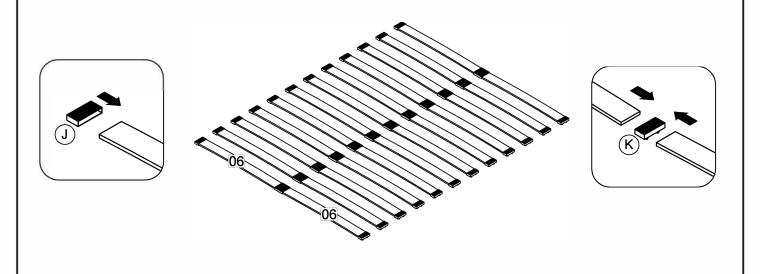
**Step 8:** Assemble hardware J and K onto mounting position on metal center bar (8), bed side (4) and (5) by using hand.
