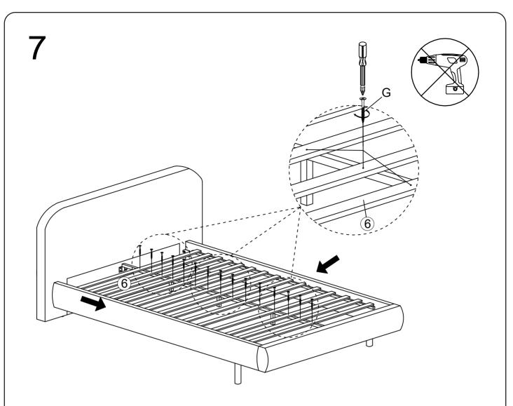
Attach the slat by pushing the side rail together so that the slat is flush against the side rail, before inserting the screw.
