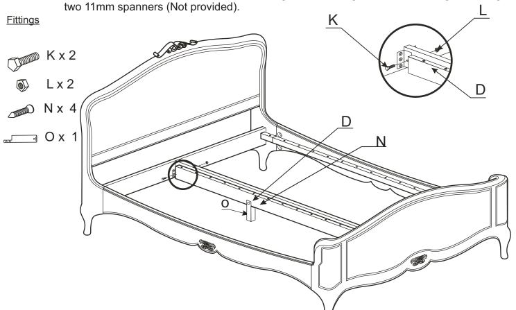
Step 6 - Push fit two plastic caps onto either end of the slat. Push fit the slat into the pre-drilled pilot holes. It may help to push the slat flat and lightly tap the plastic cap with a soft hammer. Repeat this step with the remaining slats. The assembly is now complete.
