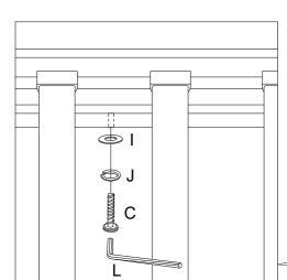
Check that the frame is central by adjusting the alignment of the frame and brackets before fully tightening all bolts. The metal frame should not contact the faux leather at any point.
