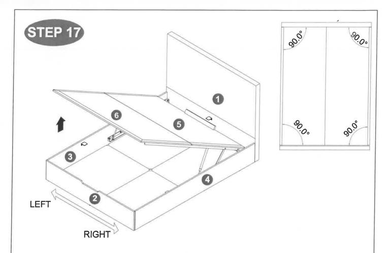
~ Make sure the Bed Frame 4 side angles are at 90 degrees before you closing the lift base.
