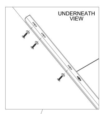
Place lift base (8) on top of mechanisms and attach as per base (7)
