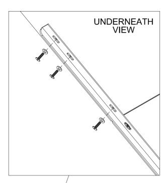
Place lift base (6) on top of mechanisms and attach as per base 5.
