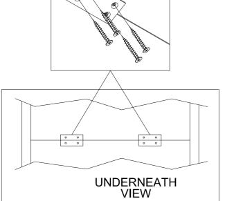
Affix metal plates to the underside of the mattress bases with fixings and screwdriver provided.
