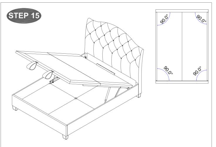
$\sim$  Make sure the Bed Frame 4 side angles are at 90 degrees before you closing the lift base.
