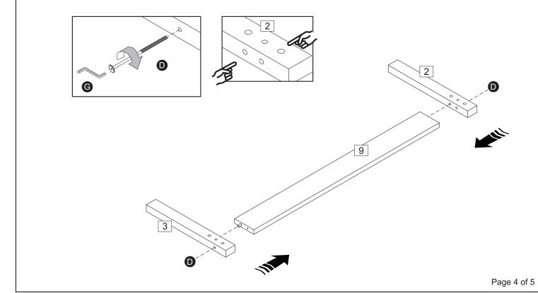
**Step 6**: Attach the side rails to the headend posts at the same time using hardware parts E, F and G. Vendor: S000238 **DO NOT use any power tools as this may damage the frame and will invalidate any claim.**
