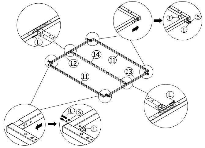
**Step 8**: Attach hardware parts **J** and **K** using hardware part **L**. **Important note: Please assemble follow arrow direction.**
