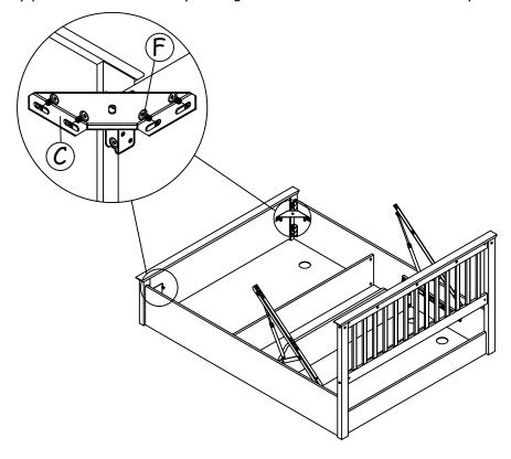
**Step 7**: Join together all the bed base parts (11),(12),(13) and (14) by using hardware parts **L,S,T**. **Important note: Please assemble follow arrow direction.**
