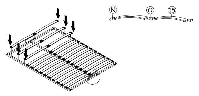
**Step 10**: Assemble the bed base on the right & left hydraulic frame and fix bolts  $\bf M$  starting from ' 10.1 ' to ' 10.3 ' as shown and stick it the self adhesive  $\bf U$  as shown.
