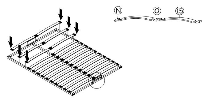
**Step 10**: Assemble the bed base on the right & left hydraulic frame and fix bolts **M** starting from '10.1' to '10.3' as shown and stick it the self adhesive **U** as shown.
