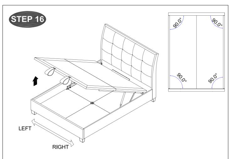
~ Make sure the Bed Frame 4 side angles are at 90 degrees before you closing the lift base.
