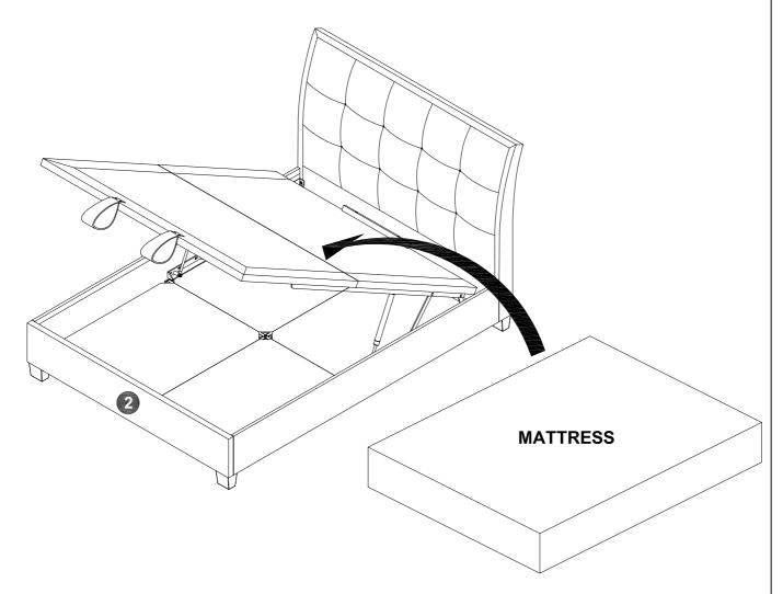
A. This Lift Mechanism provides assistance with the lift of the mattress fitted to the base - it does not lift the mattress for you. The system has been designed to effectively lift the base system fitted with a variety of mattress weights and combinations of depth. The combination of mattress weight and depth determines the degree of assistance provided by the mechanism.
