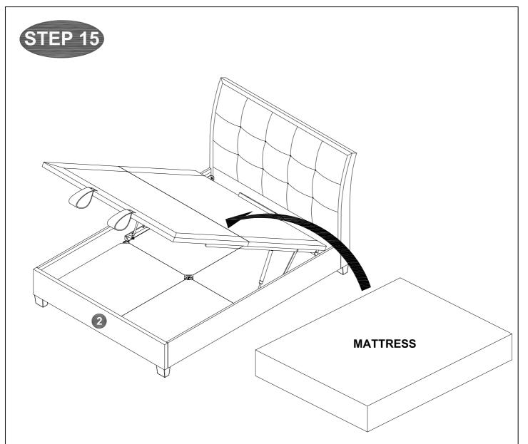
A. This Lift Mechanism provides assistance with the lift of the mattress fitted to the base - it does not lift the mattress for you. The system has been designed to effectively lift the base system fitted with a variety of mattress weights and combinations of depth. The combination of mattress weight and depth determines the degree of assistance provided by the mechanism.
