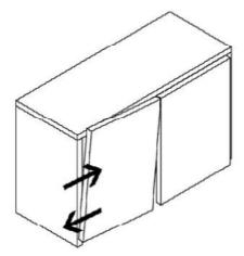
Lateral Adjustment by adjusting screw
