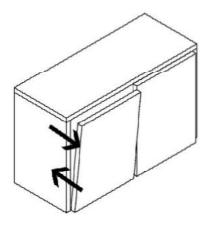
**Depth Adjustment** after loosening the hinge arm mounting screw
