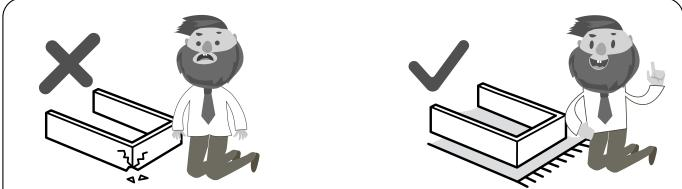
Never drag or push the pieces across a hard or stone floor as this will cause damage to the joints. Use a carpet or a rug for extra care.
