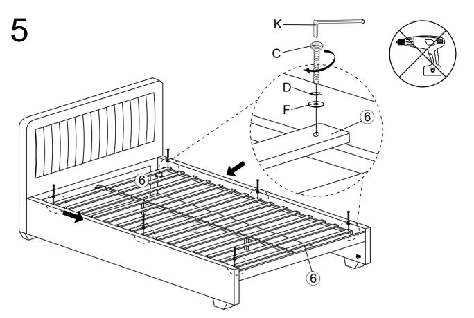
Attach the slat by pushing the side rail together so that the slat is flush against the side rail, before inserting the screw.
