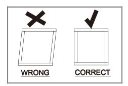
3 Fix corner brackets, then repeat for other 3 corner brackets in each corner of the bed frame.
