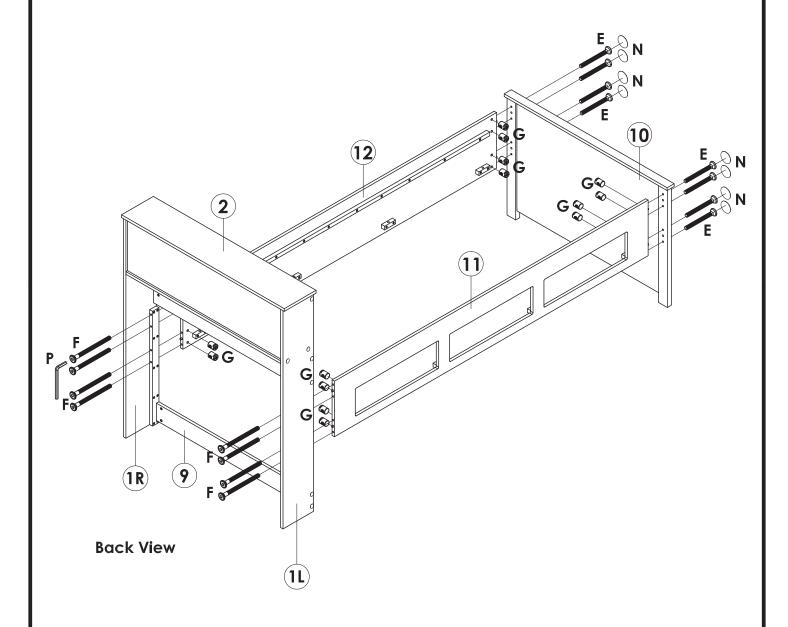
Attach and Secure **Side Rail (Left)** and **Side Rail (Right)** onto **Headboard** by using **(F)** and **(G)**,onto **Footboard** by using **(F)** and **(G)** tighten it up by using **(P)**. Follow it up by attaching **(N)** into screw holes.
