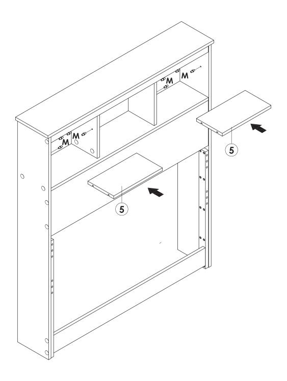
Insert (M) into Ø5MM holes on Side Panel L&R (Headboard) and Divider (Headboard).
