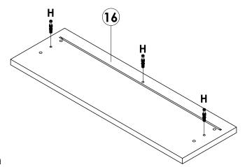
Insert **(H)** into Ø5MM holes on **Drawer Face** by using crosshead screw driver.
