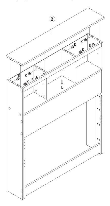
Attach and Secure **Top Panel (Headboard)** onto **SIde Panel L&R (Headboard)** by using **(K)** and **(L)**, tighten it up by using Crosshead screw driver.
