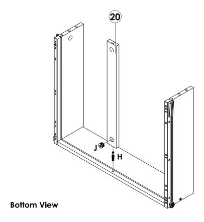
Attach and Secure **Drawer Support (Base)** onto **Drawer Rear**,by using **(H)** and **(J)**, tighten it up by using crosshead screw driver.
