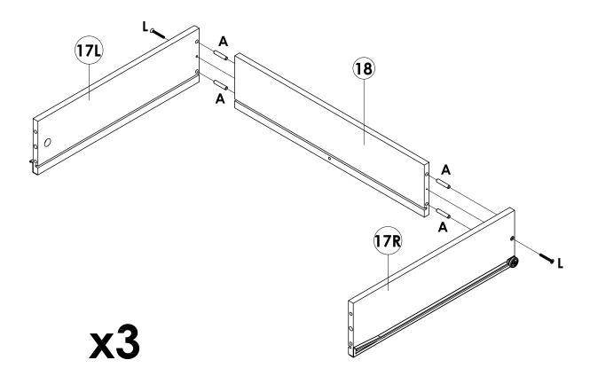
Attach and Secure **Drawer Side (L/R)** onto **Drawer Rear**, by using **(A)** and **(L)**, tighten it up by using crosshead screw driver.
