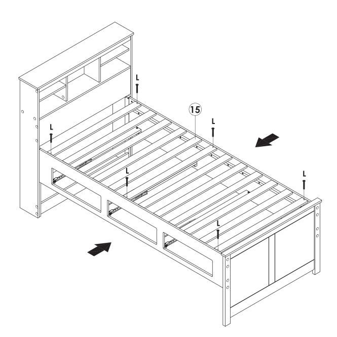
Attach and secure **Wooden Slat** onto bed **Slat Support** by using **(L)**, tighten it up by using a Crosshead Screw Driver.
