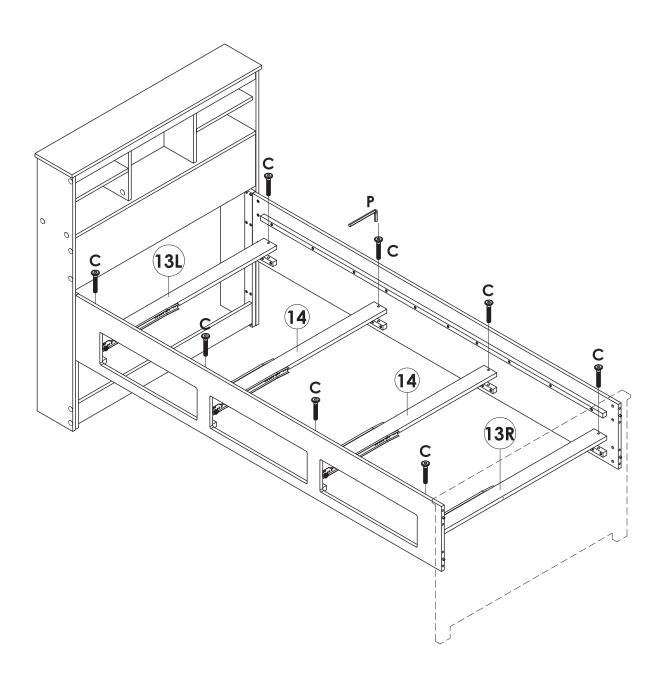
Attach and Secure **Drawer Support Side (L/R)** and **Drawer Support (center)** onto **Side Rail (Left)** and **Side Rail (Right)** by using **(C)**, tighten it up by using **(P)**.
