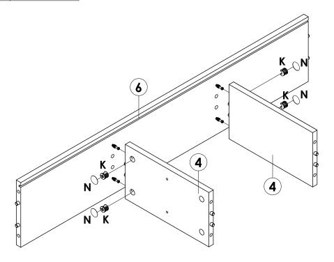
Attach and Secure **Divider (Headboard)** onto **Bottom Shelf (Headboard)** by using **(K)**, tighten it up by using Crosshead screw driver. Follow it up by attaching **(N)** into screw holes.
