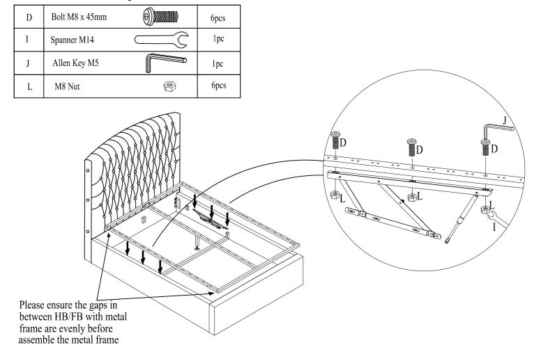
DO NOT use any power tools as this may damage the frame and will invalidate any claim.
