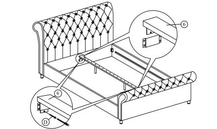
Step 5: Attach the slats (5) using hardware parts E and F then secure the bolts using hardware part C. **DO NOT use any power tools as this may damage the frame and will invalidate any claim.**
