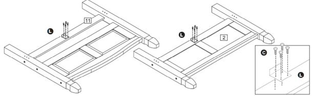
Step 6: Attach the side rails (9) using hardware parts J, K and M. Secure the centre rail (10) using hardware parts E and F.
