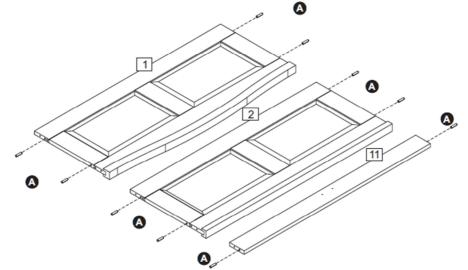
**Step 3:** Attach the left headend post (3) and right headend post (4) to the headend panel (1) and headend rail (11) using hardware parts H and M.
