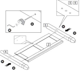
Step 5: Secure hardware part L using hardware part C and a screwdriver (not provided). DO NOT use any power tools as this may damage the frame and will invalidate any claim.
