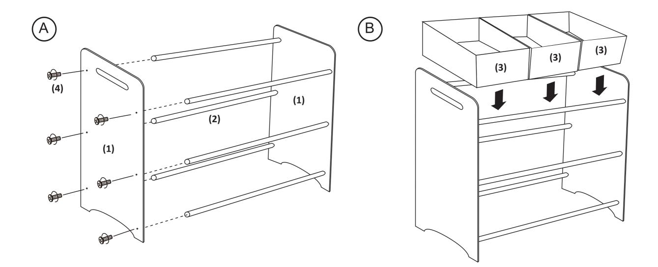
A. Take a side panel (1) and screw in the front/back poles (2) with the screws (4) supplied. Repeat this with the other side panel (1).
