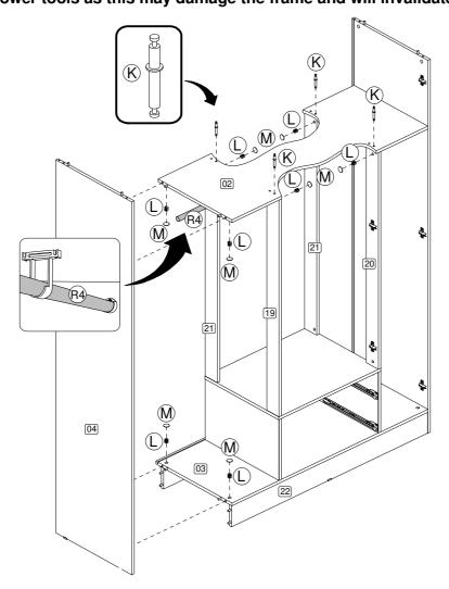
**Step 8:** Attach the shelf dividers using hardware parts L and M with a screwdriver (not provided). Connect two back panels (23) together with the spine (A6) and position.
