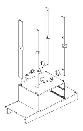
**Step 6:** Attach the right panel (8) and shelf (2) using hardwareparts L and M and a screwdriver (not provided). **DO NOT use any power tools as this may damage the frame and will invalidate any claim.**
