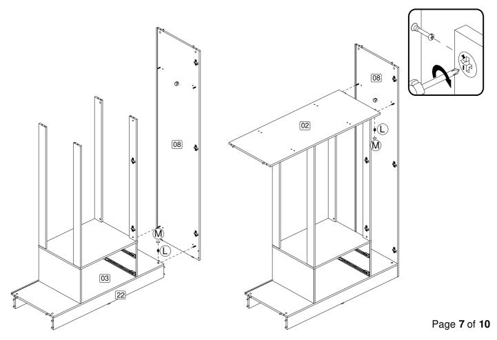
**Step 7:** Secure the shelf (2) to the supports using hardware parts L, M and K. Position the hanging rain (R4). Attach the left panel (4) using hardware parts L and M. You will need to use a screwdriver (not provided). **DO NOT use any power tools as this may damage the frame and will invalidate any claim.**
