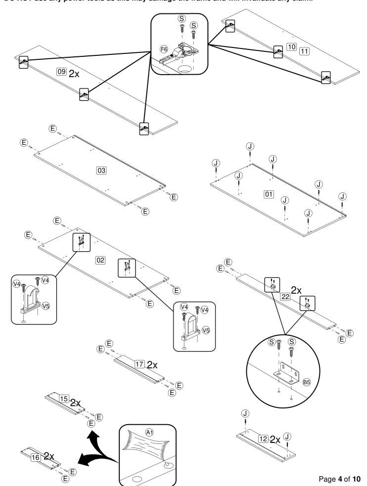
**Step 1:** Prepare these parts for assembly using hardware parts D5, E, E7, F, J, N, P5, S, WA, WB and Z4. You will need to use a small mallet and a screwdriver (not provided).
