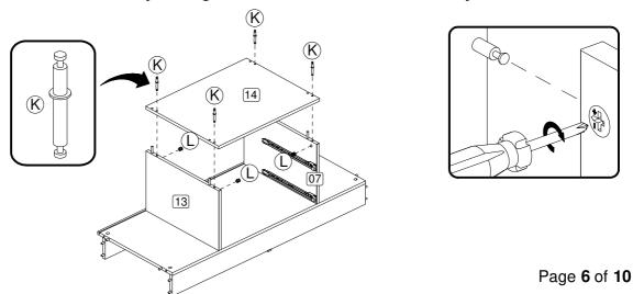
**Step 5:** Attach the supports using hardware parts L and M with a screwdriver (not provided). **DO NOT use any power tools as this may damage the frame and will invalidate any claim.**
