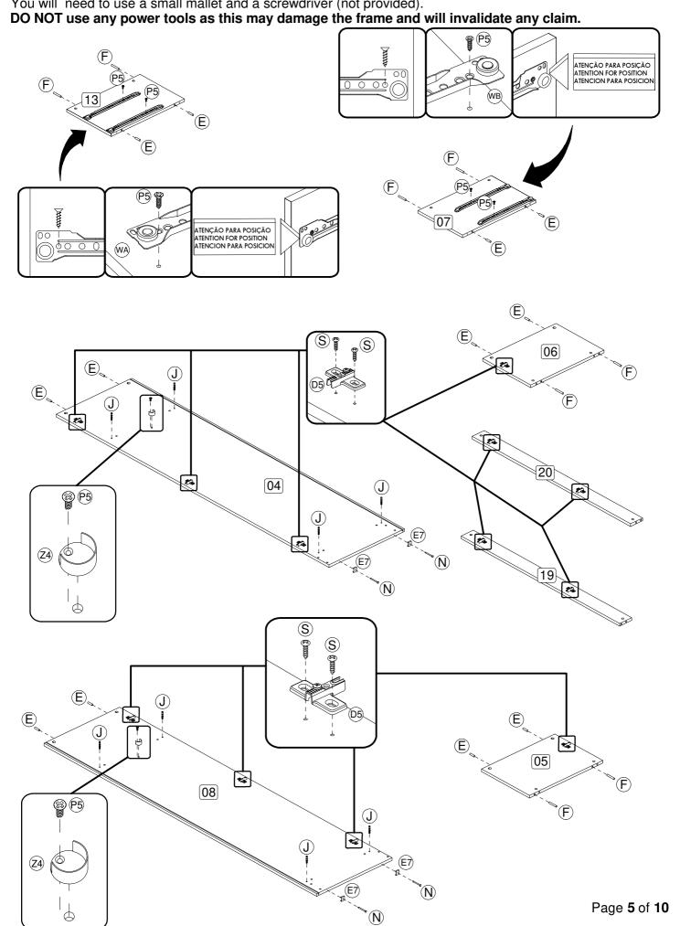
**Step 2:** Attach the drawer cabinet right panel (7) and darwer cabinet left panel (13) to the base panel (3) using hardware part O and a screwdriver (not proveded).
