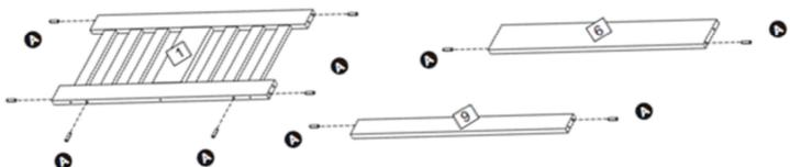
**Step 3:** Attach the right headend post (2) and left headend post (3) to the headend panel (1) and headend rail (9) using hardware parts E and H.
