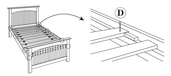
Step 3: Attach the trundle endboard (P5) to the trundle side rail (P6) using hardware parts F, H, I and J. DO NOT use any power tools as this may damage the frame and will invalidate any claim.
