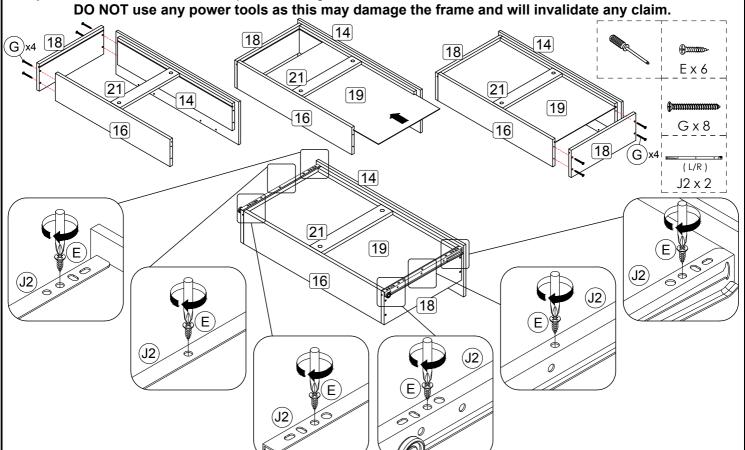
Step 11: Assemble the drawer components using hardware E, G and J2.
