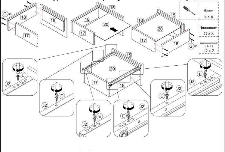
Step 12: Assemble the drawer in place along the drawer slides.
