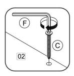
Step 5: Attach the Metal Middle (11) to panel (2) using hardware I and F.
