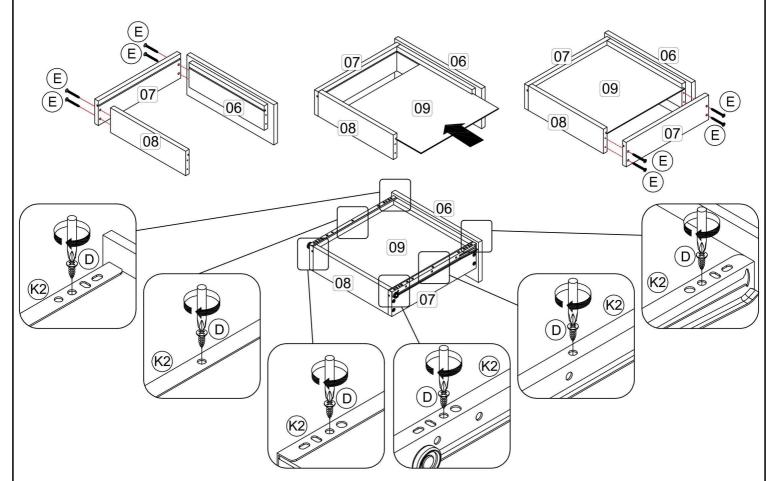
Step 9: Assemble the drawers in place along the drawer slides.
