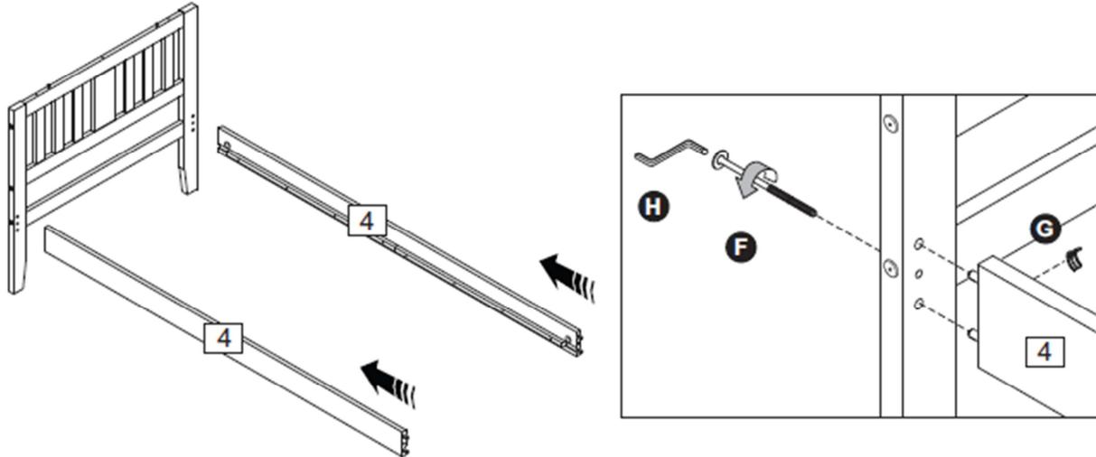
Step 6: Attach the footend using hardware parts F, G and H.
