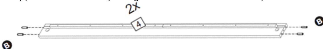
Step 2: Insert hardware part A to the headend panel (1), footend panel (6) and headend rail (9) using a small mallet (not provided).
