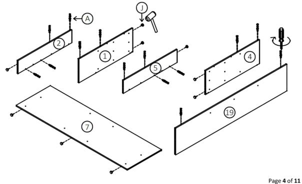
Step 3: Join the end panels together as shown using hardware parts A, B and K DO NOT use any power tools as this may damage the frame and will invalidate any claim
