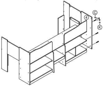
Step 18: Secure the right back post (23) and left back post (22) using hardware parts A, B, C and K. DO NOT use any power tools as this may damage the frame and will invalidate any claim
