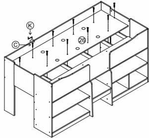
Step 21: Insert hardware parts L.
