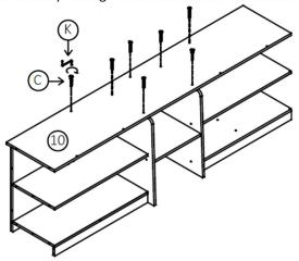
Step 15: Attach the left front panel (20) and right front panel (21) using hardware parts C and K. DO NOT use any power tools as this may damage the frame and will invalidate any claim
