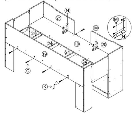
Step 20: Attach the back base panel (26) using hardware parts C and K. DO NOT use any power tools as this may damage the frame and will invalidate any claim
