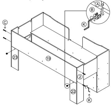
Step 19: Secure the support plinths (24) using hardware parts C and K. Attach hardware part N using hardware part M and a screwdriver (not provided).
