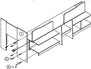
Step 17: Attach the assembled right end panel using hardware parts C and K. DO NOT use any power tools as this may damage the frame and will invalidate any claim
