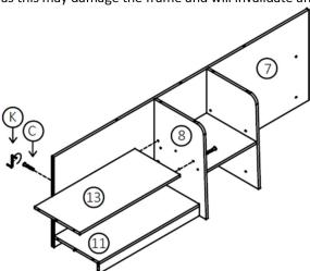
Step 11: Attach the right lower shelf panel (12) and side front plinth (18) using hardware parts C and K. DO NOT use any power tools as this may damage the frame and will invalidate any claim
