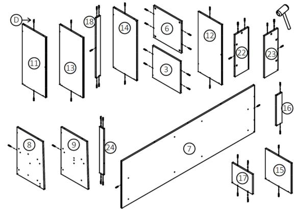
Step 2: Insert hardware part J using a small mallet (not provided). Insert hardware part A using a screwdriver (not provided)
