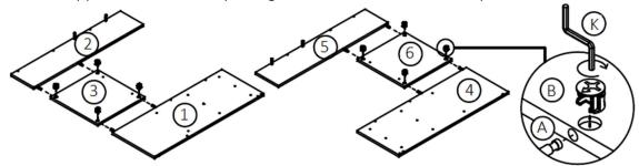
Step 4: Fix the left back post (22) to the left back end panel (2), and the end support (25) to the left centre end panel (3) using hardware parts A, B and K. Repeat for the right back post (23), right back end panel (5) and right centre end panel (6).
