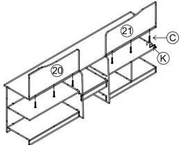
Step 16: Attach the assembled left end panel using hardware parts C and K. DO NOT use any power tools as this may damage the frame and will invalidate any claim
